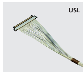
[Cable bundling] Bundle of partial tapes
