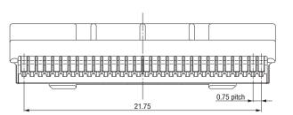
X-X' Cross Section (With the contact inserted)
